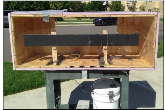
(Single louvre test bed used to validate theoretical models by UST student researcher, Elvis Popov.)
