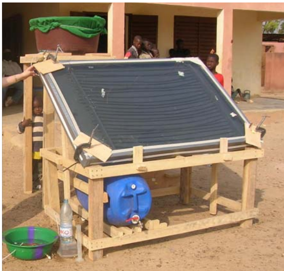
Left: Working prototype in Mali, West Africa. Above: A CAD drawing of final design recommendation for water pasteurizer.
