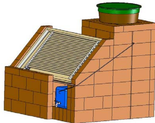
Left: Working prototype in Mali, West Africa. Above: A CAD drawing of final design recommendation for water pasteurizer.
