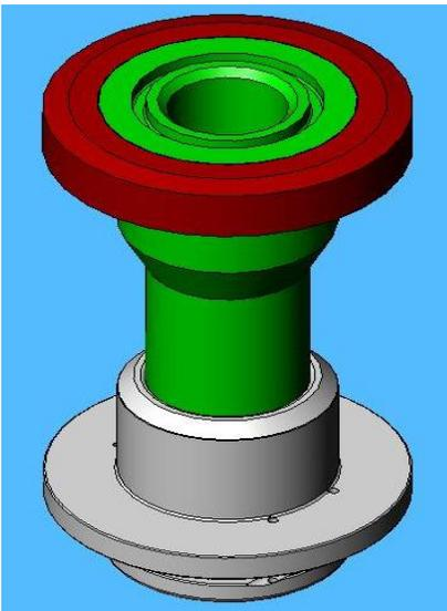
SolidWorks drawing of the final design canister assembly.
